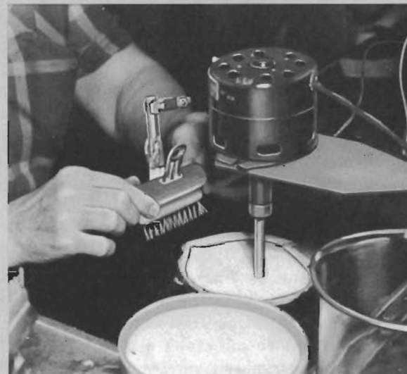
Heater failures due to excessive intermittent operation are virtually eliminated in G-E Five-Star tubes by the use of heavier heater wire and careful control of coating process. The bends in Five-Star heater wire are specially coated a second time with the help of an electrical charge that deposits material wherever the coating may have cracked off during formation of the heater.
