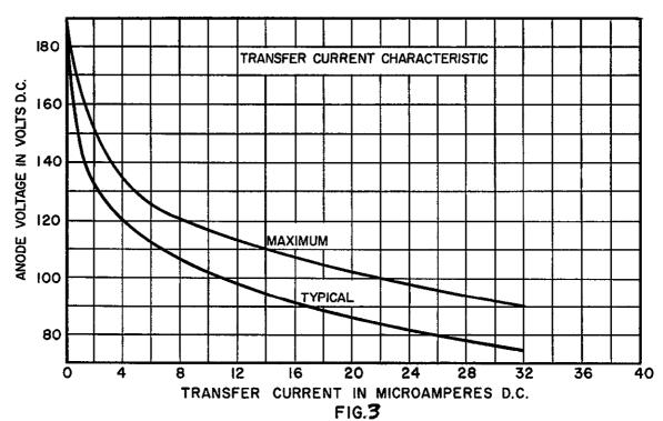
Note 3: Limits apply immediately after the tube has conducted current. If tube has been idle, these values initially may be as much as 3 volts higher or lower.
