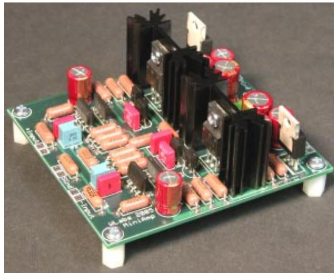
As usual, with all Welborne Labs kits, we offer several options including: with or without the on-board voltage regulators, kit or assembled, and upgrade options featuring the super low noise Caddock foil resistors, ELNA Cerafine capacitors and the low noise Linear Technology voltage regulators. We suggest you mate a couple of the MINI AMPS with our PS5 dual-mono power supply kit and you will end up with a killer linestage that'll enhance ANY system.... tube or solidstate!
