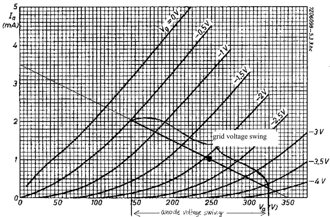
Again the working line is drawn for  $V_{\text{supply}} = 350V$  and  $R_{\text{load}} = 100k\Omega$ . The Working point is marked with a dot and the maximum usable part of the line is bold.
