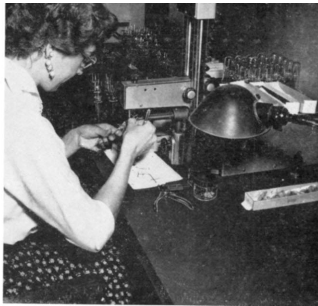
Second step: (above) Assembling the cathodes in vacuum tubes.
