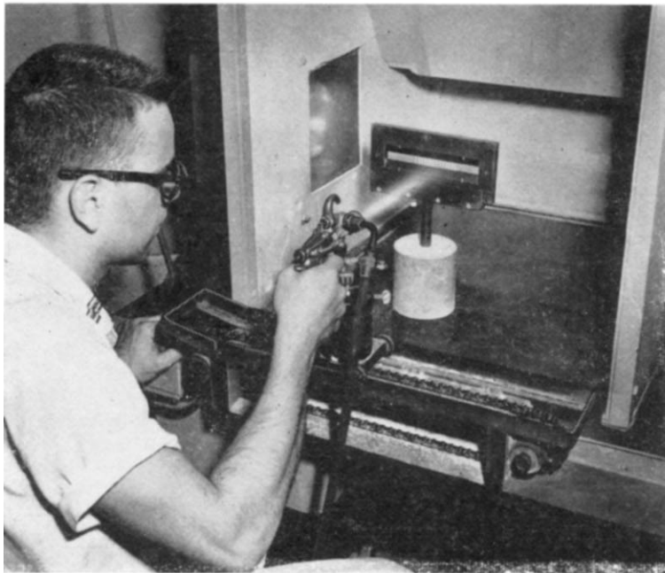
First step: Spraying the cathodes with a coat of barium-strontium-calcium-carbonate.
