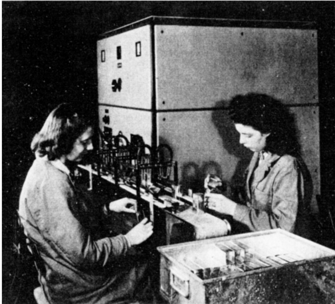
Fig. 18-14. High frequency soldering of capacitor housings.
