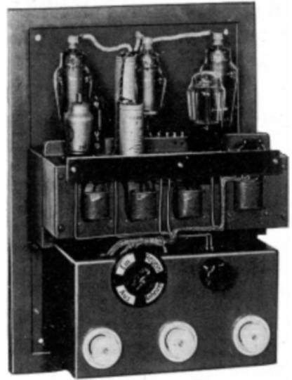
Fig. 15-16. Electronic temperature regulating device for heating powers up to 1.5 kW.
