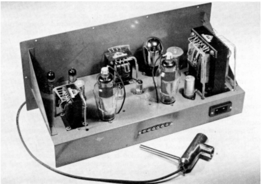
Fig. 15-7. Experimental equipment corresponding to the circuit of fig. 15-5.
