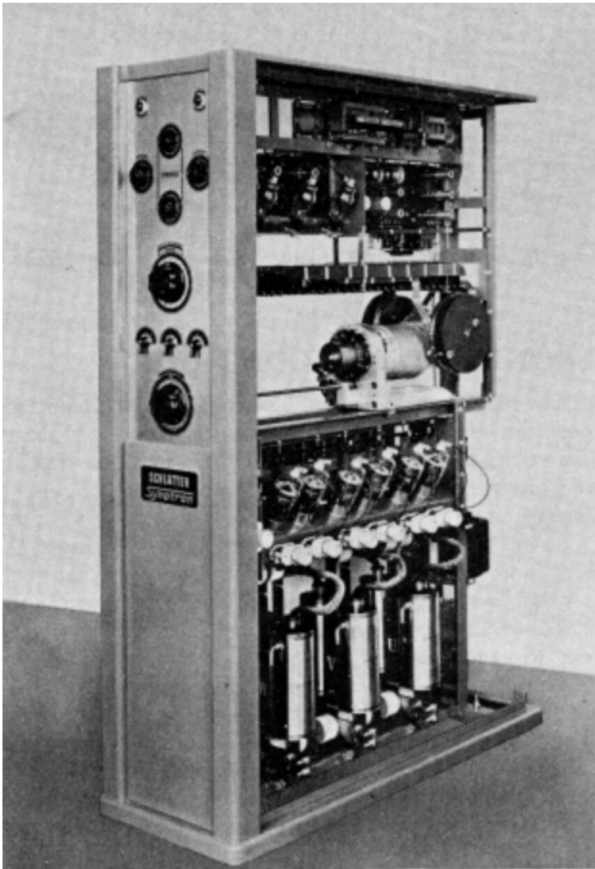
Fig. 16-21. Three-phase welding equipment.
