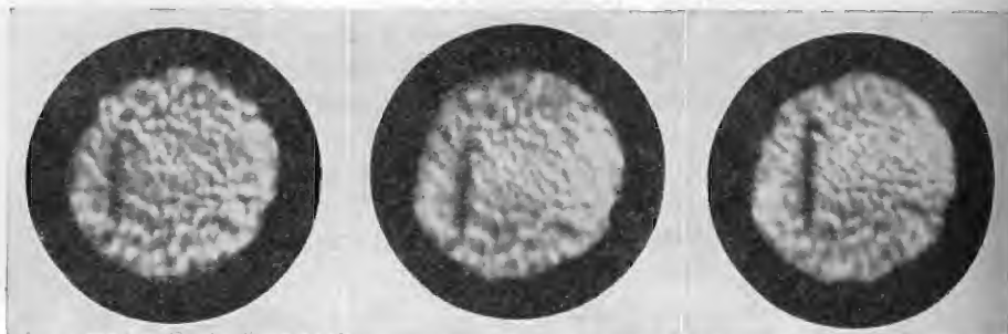
Fig. 99.—Electron Images of an Oxide Cathode taken during Further Activation (mag. \times 30 ): (a) I_s = 10^{-6} amp.; (b) I_s = 2 \times 10^{-3} amp.; (c) I_s = 2 \times 10^{-2} amp. (Heinze and Wagener 2 ).
