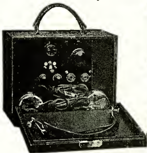
Model P-12 Two Tube Portable. Model P-11 with amplifier tube added, which increases distance and volume many times. $22.50.
