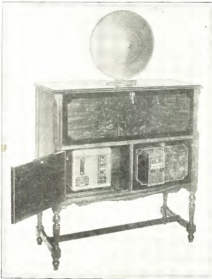
Photo A. View of receiver mounted in console, with suggested accessories
