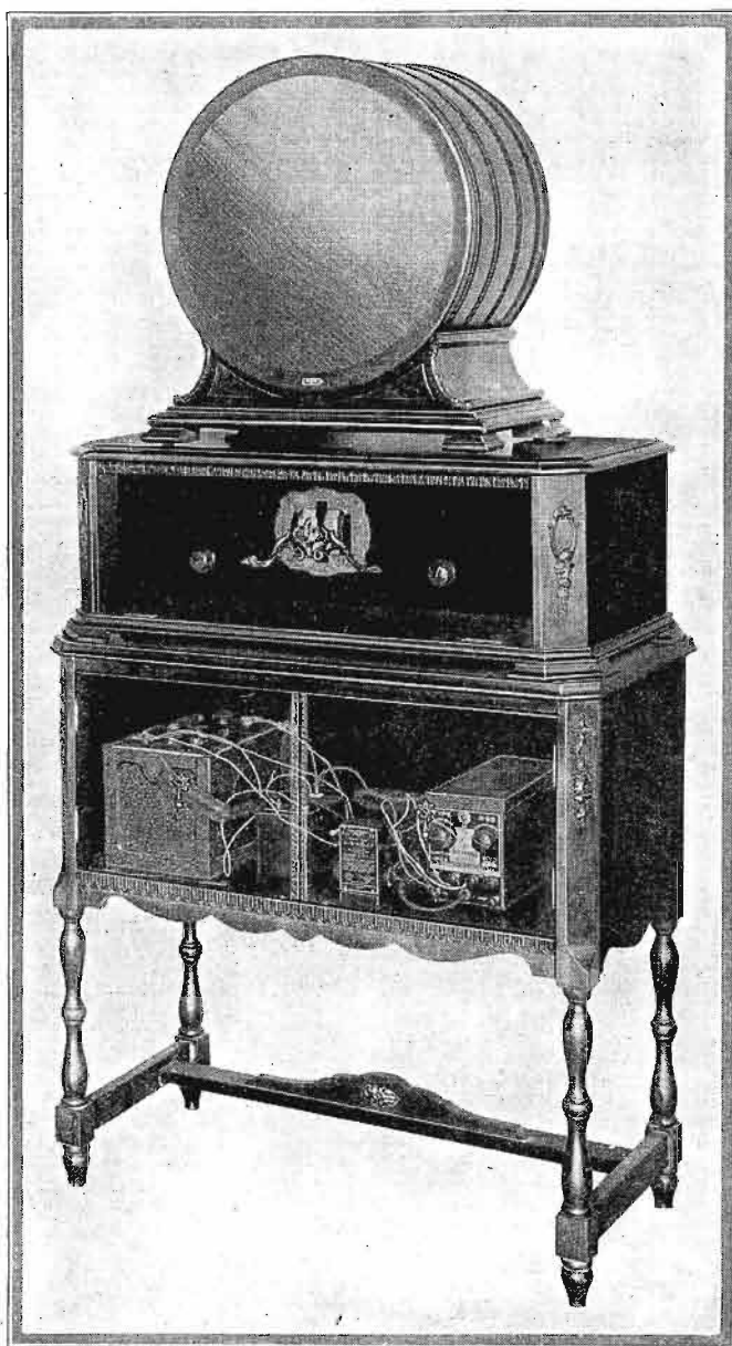
Photo A—Suggested assembly of Tyrman Ten with loudspeaker and accessories
