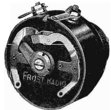
FROST-RADIO DE LUXE VARIABLE HIGH RESISTANCES WITH SWITCH Construction is identical with Series 1880-1890 Resistances except that filament switch, mounted on Bakelite panel, operates when knob is turned to left, locking in "off" position. Nickel silver springs have sterling silver contacts. 2,000 to 500,000 ohms. Series S-1880, 2 terminals . . . . . $2.10 Series S-1890, 3 terminals . . . . . $2.10
