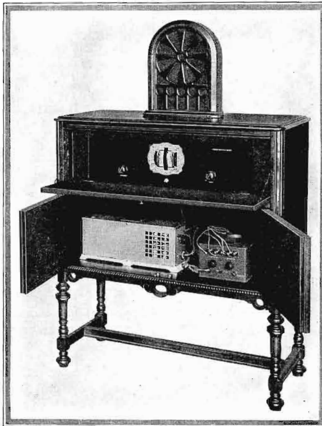
View of completed receiver installed in a console with suggested accessories
