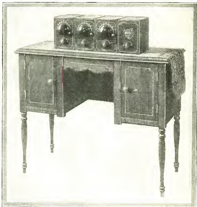
Figure 1. Front view of Vari-units shown on console table. Quite a number of combinations may be made by merely adding sections to the basic receiver
