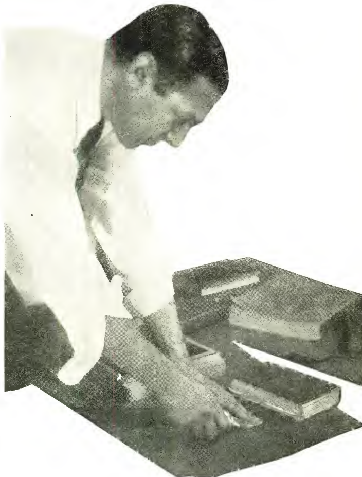
Figure 3. In making the G. R. P. speaker the back cone is weighted. With one finger preventing the cement from seeping between the cones, apply the Ambroid cement around the circumference of the back cone
