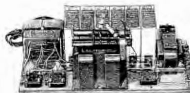
Figure 2. The power supply used with the Victoreen receiver is shown in the above photograph
