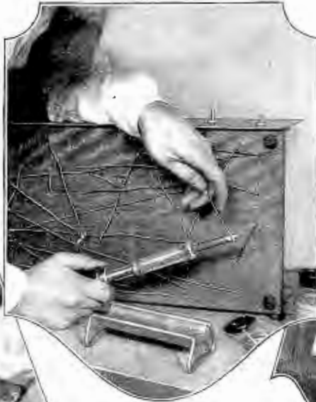
Wiring Without Solder Lugs
