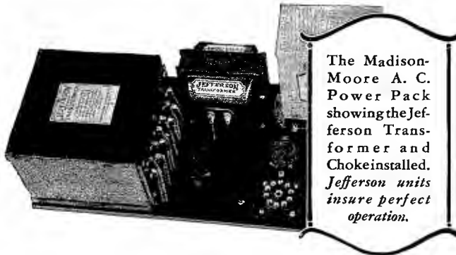
Jefferson Combination Filament and Plate Supply Transformer No. 463-101 for use with Madison-Moore A. C. International "One-Spot."
