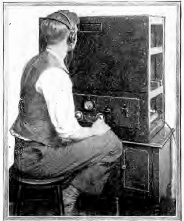
Fig. 2. This photograph shows the scanning mechanism and housing used at present in the laboratory for local television reception. The operator is wearing a pair of Frost head phones and monitors the received signal in order to catch any voice announcements that may be made during the program. The meter on the panel is in series with the television lamp, in order to tell when more than its rated current is being used
