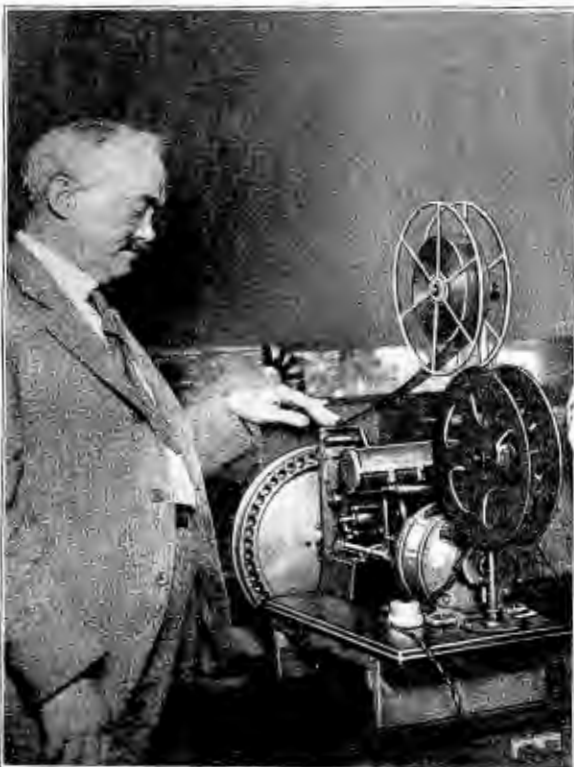
Fig. 1. Here is a photograph of the new Jenkins transmitter being used at Washington for producing radio movies and which may shortly be available to broadcast stations desiring to transmit radio movies
