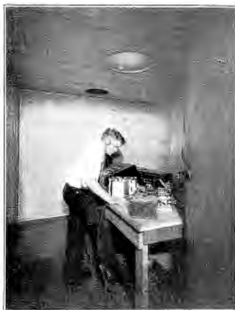
(All receivers serviced in this laboratory are given a final test in a completely shielded room where the internal noises are absolutely eliminated.) This insures noise-free reception, which is necessary for satisfactory performance. In addition, complete equipment is available for properly testing all types of power units.
