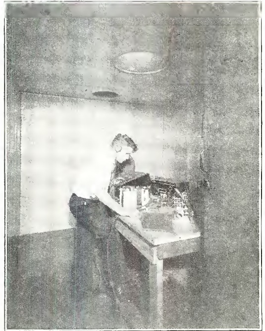
(All receivers serviced in this laboratory are given a final test in a completely shielded room where the internal noises are absolutely eliminated.) This insures noise-free reception, which is necessary for satisfactory performance. In addition, complete equipment is available for properly testing all types of power units.
