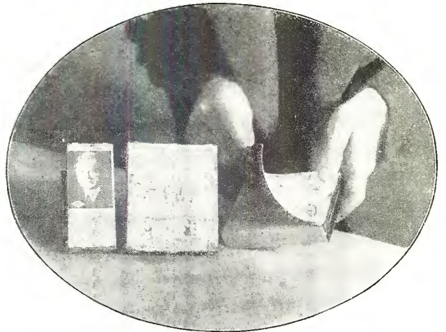
A new plate, taking the place of the mat and the electrotpe, has made its appearance on the market, and all signs point to its revolutionizing the printing industry. The invention consists of a flexible plate, fabricated by a special process from a paper base so light that it can be whisked through the mails as first class matter, and yet withstand wear and tear and general knock-about handling to a degree that metal plates can not endure. The new paper plate is capable of being run off on either the flat bed or cylindrical presses, without mechanical make-ready. It is the invention of Fred C. Goldenbaum of New York. Photo shows three of the newly invented paper plates mounted on blocks ready for flat bed presses
