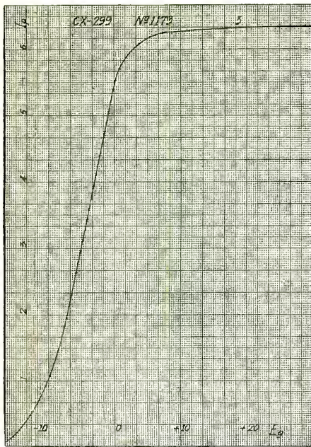
Fig. 2. In the graph is shown an E_g-I_p curve of a 199 tube. By examining the graph, it will be noted that from 0 to 10 negative E_g the I_p makes a decided rise and from 10 plus up the current I_p increases very little with a large increase of E_g . This is called saturation. That means the filament is emitting all the electrons possible, making the space between the plate and filament saturated
