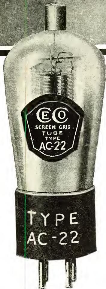
The screen grid tube using the separate heater principle and requiring 1.75 amps at 2.5 volts.
