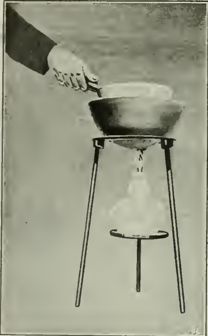
Fig. 1. Apparatus Used in Making Test for Butter and Oleomargarin or Renovated Butter.
