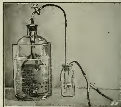
Completely Assembled Gas Generator and Wash Bottle.
