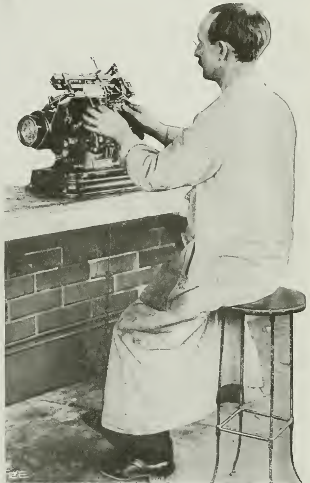
Wherever Good Shoes Are Made—There Also Shoes Must Be "Laced" Before Being "Lasted." Once, Skilled Humans Performed This Job; Now a Machine Does It—Accurately and Quickly.
