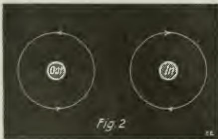
To Produce a "North" Magnetic Pole, the Current Must Pass Counter-clockwise Around the Core as Shown at the Left. A "South" Pole Results from a Clockwise Direction of Current Thru a Magnet Coil.
