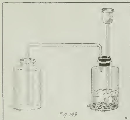
Apparatus for Generating Hydrogen Sulfid By the Action of Hydrochloric Acid on Ferrous Sulfid and the Collection of the Gas by Downward Displacement.
