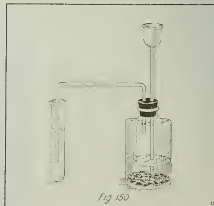
The Apparatus Employed for "Precipitation" By Hydrogen Sulfid.
