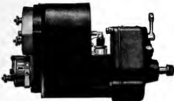
By Storing Up Energy in a Special Spring Coupling Device, It Becomes Possible to Spin This Magneto at Starting, and Provide a Hot Spark.
