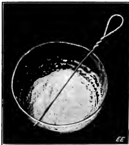
A Small Silica Capsule, Shown in Natural Size, Containing 1.764 Milligrams of Anhydrous Radium Barium Bromid, Having a Radium Element Content of 740 Milligrams. At the Present Market Price of $120 Per Milligram, This Radium Shown in the Dish Has a Cash Value of $88,800.
