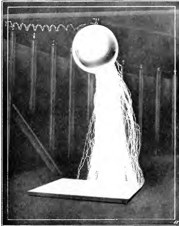
Fig. 2—This illustrates tests with spark discharges from a ball of forty centimeters radius in Tesla's Wireless Plant erected at Colorado Springs in 1899. The ball is connected to the free end of a grounded resonant circuit seventeen meters in diameter. The disruptive potential of a ball, is, according to Tesla, in volts approximately V = 75,400 r ( r being in centimeters). That is, in this case 75,400 \times 40 = 3,016,000 volts. The gigantic Tesla coil which produced these bolts of Thor was capable of furnishing a current of 1,100 amperes in the high tension secondary. The primary coil had a diameter of 51 feet! This Tesla coil produced discharges which were the nearest approach to lightning ever made by man.
