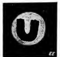
Radiograph Taken by the Author, Using An E. I. Co. Spintariscope with Lens Removed. The Figure "U" Was Cut from Brass Sheet.
