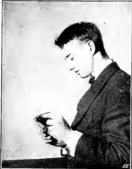
Fig. 19. The Burning Test Applied to Various Cloth Materials to Determine Their Composition, Particularly the Presence of Wool. Vegetable Fibers May Be Readily Distinguished from Animal Fibers By Burning, Animal Fibers Such as Silk and Wool Giving Off the Smell of Burnt Horn. They Do Not Burn Like Vegetable Fibers, But Cease to Burn When Removed from the Flame. Vegetable Fibers Give Off a Slight Odor of Burnt Wood When Ignited, and They Burn Away Very Rapidly With a Flash, leaving No Hard Cinder, But a White or Gray Ash Only.
