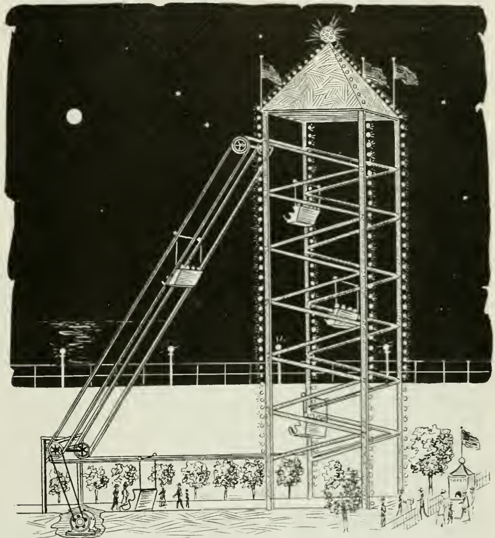
The Latest Electrically Operated Thriller for Pleasure Resorts is Known as the "Zig-Zag." The Passengers Are Hauled to the Top of the Tower by a Motor-driven Cable. They Then Start Their Zig-Zag Downward Journey by Gravity.
