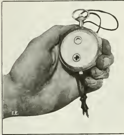
A Watch Style Polarity Indicator of the Magnetic Type Appeals to Every Electrical Man. Details for Making One Are Given Herein.
