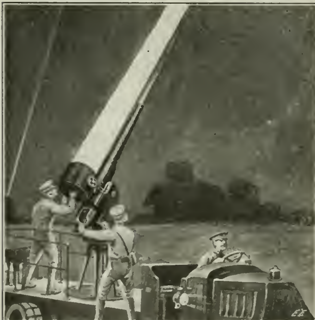
English Anti-Aircraft Guns Used in the Aerial Defense of London Have Been Fitted With Searchlights to Increase the Accuracy and Rapidity of Fire, This Unit Being Mounted on a Motor Truck.
