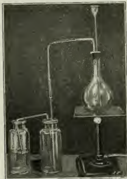
Fig. 133. Set-Up of Chemical Apparatus for Preparing Chlorin Gas From Hydrochloric Acid and Manganese Dioxid.
