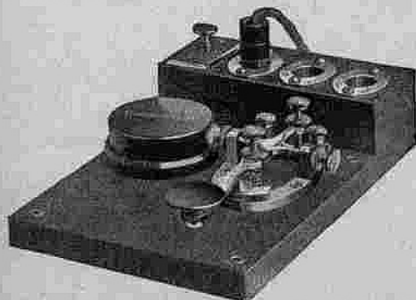
A Code Teaching Instrument Provided With Plug Switch for Battery and Omnigraph.
