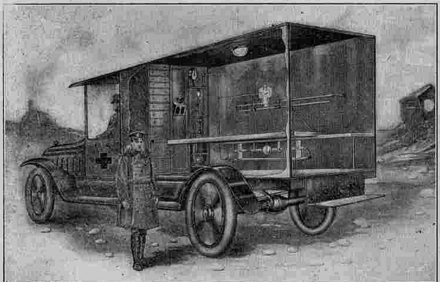
The Latest Design of Portable X-Ray Ambulance for U. S. Army. It Derives Its Power, About Two Kilowatts, from a Special Dynamo Driven by the Engine. It Includes Plate Developing Facilities, Complete Switch-Board for Controlling X-Ray Bulbs, and Other Necessary Conveniences.
