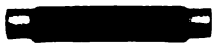
Ward Leonard vitrohm resist-ance units for filament current adjustment and other uses. The best obtainable. Absolutely constant resistances—5 ohms with ferrules, 7 1/4" x 3/4", 90c; 60 ohms, no ferrules, 2" x 3/4", 65c; 90 ohms with ferrules, 2" x 3/4", 75c; 5000 ohms, graphite sectors, 2 1/2" x 3/4" x 1/4", for adjustable grid leak resistance, 55c.
