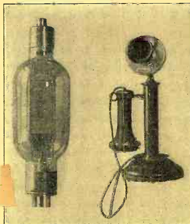
Fig. 3. Comparison of Size Between a 1 k.w. DeForest Oscillation Tube and an Ordinary Desk Telephone. Two of the ½ k.w. Type Were Used in the Experiments.
