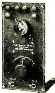
Vertical Panel-style mounting, without cabinet. Two legs hold each panel upright. Any number of panels may be joined and mounted this way.
