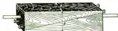
The Windings of the Transformer Are Made on a Form of This Type Before Being Mounted on the Core.
