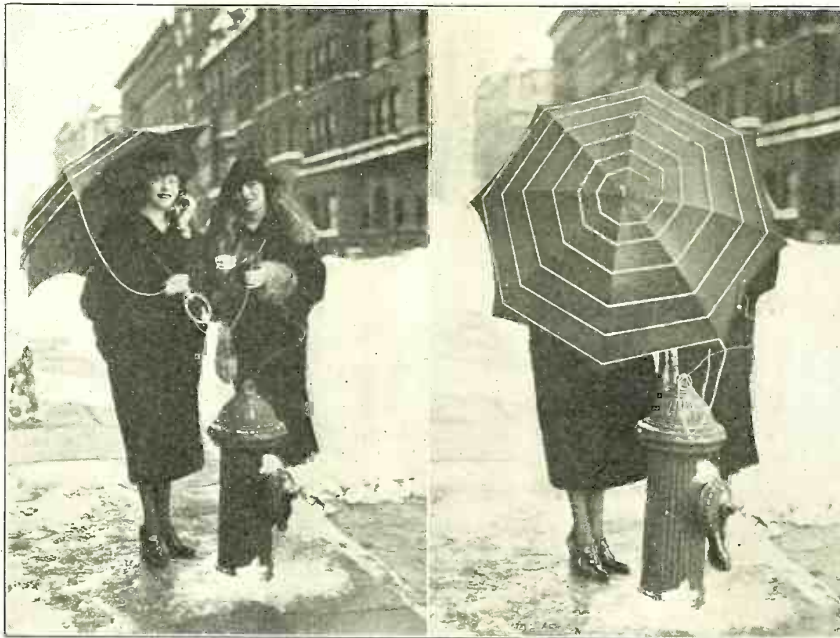
This Photograph Shows the Latest in Portable Radio Sets. The Aerial is Sewed on an Umbrella and a Hydrant is Used as a Ground as Shown in the Right Hand Photograph. On the Left is a View of the Two "Ops" Listening in to a Fone Conversation While Out For a Walk. These Two "Ops" are Miss Peggy and Alice Brady, of the Ziegfeld Midnight Frolic.
