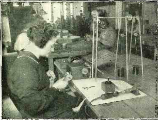
Left: These Machines Wind a Complete Bobbin in Less Time Than It Takes to Tell It; 3,500 Turns of Wire Per Minute Are Put in Place. A Special Counting Device Tells the Operator When the Proper Number of Turns Are Placed. Right: This Expert Mechanic Is Grinding the Pole Faces of the Magnets. Great Care Must Be Taken as the Removal of a Hairbreadth of Metal Too Much, Seriously Affects the Receiver's Operation.
