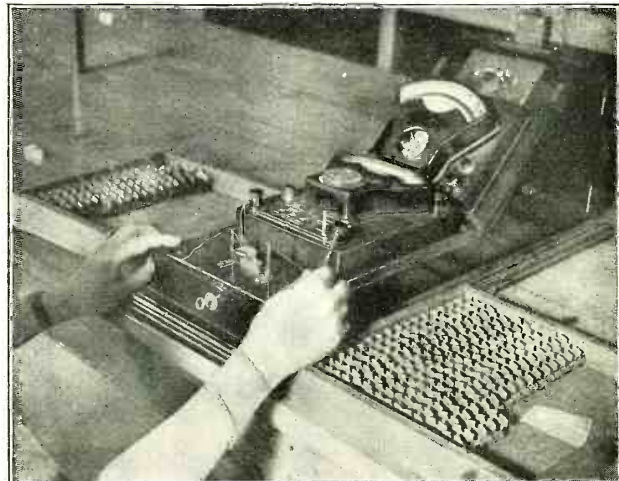
This Machine Measures the Resistance of the Bobbins and Tells Whether or Not the Winding is Grounded. The Resistance is Read Directly Off the Scale. It is the only Machine of its Kind.
