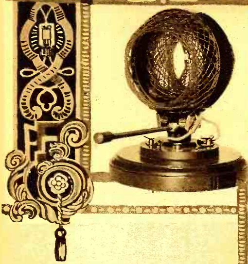
Top Left: A Seven-Tube Receiving Set of English Design. The "B" Battery and Loud Speaker Are Seen in the Interior of the Cabinet. Top Right: An English Set of the Desk Type. When Closed, it Resumes an Upright Position. Left: A Variometer With Windings Similar to Those of the Honeycomb Coil. Variation is Accomplished by a Handle Protruding From the Base of the Instrument.
