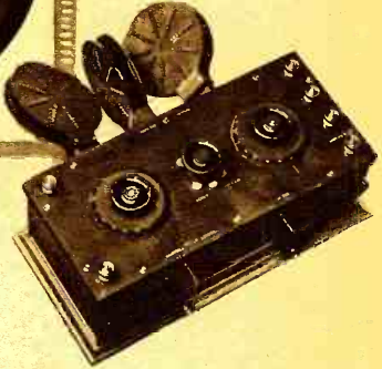
Left: A fixed inductance coil of the multi-layer type with plug attachment. An air space is left between each layer similar to the Morecroft inductance. Below: A small receiving set employing three of these coils.
