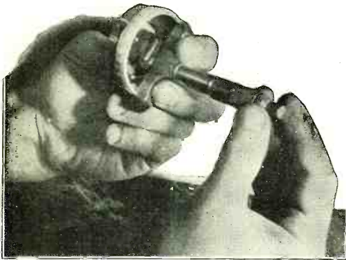
Here We See How the Depth Micrometer Is Used in Measuring Up the Distance of the Pole Faces from the Edge of the Receiver Case.
