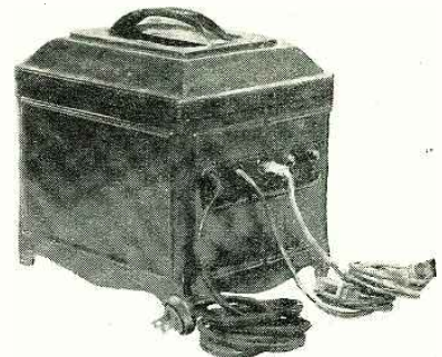
Fig. 5. The above illustration is a rear view of the charger shown at the lower left. The taps are for the purpose of varying the voltage, according to the battery to be charged. Photos by courtesy of Gen. Electric Co.
