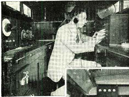
Fig. 3. (Above). An interior view of the radio detective car, which has proved very useful in locating power leaks and other forms of interference, as well as in running down violators of the radio laws.
