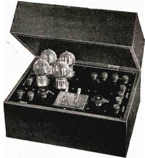
This is a Power Amplifier Used to Boost up the Current of a Microfane Circuit in Order to Operate a Telemegafone at Maximum Efficiency.
