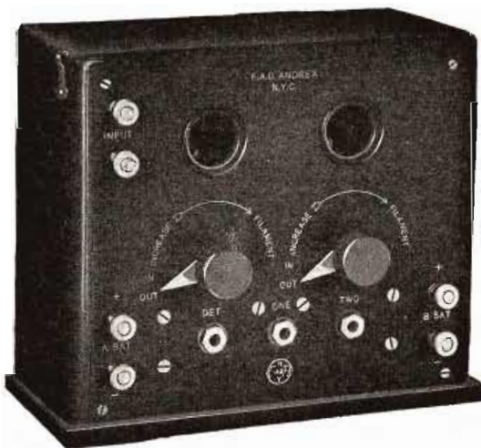
ABOVE—FRONT OF TWO-STAGE AMPLIFIER
