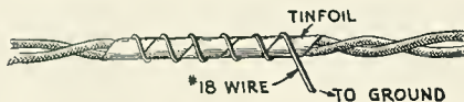
By preparing the A.C. leads to a set as shown, a great deal of the hum is stopped.
