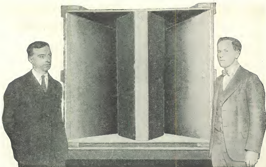
The exponential horn mounted on a pedestal, preparatory to the demonstration during which the voice of the horn was clearly heard, three-quarters of a mile away. The inventors—Dr. Slepian at the left, Mr. Hanna at the right, are shown beside it.
