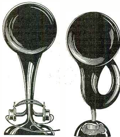
Fig. 3 (left). An early speaker which employed a pair of phones as a driving unit. Fig. 4 (right). Another early speaker, with phone unit mounted in base.
