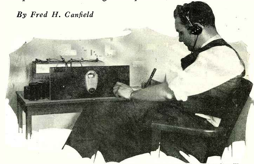
Fig. A. This picture, taken in RADIO NEWS Laboratories while testing the Screen-Grid Short-Wave Receiver, clearly shows the neat, uncluttered appearance of the front panel. The coils for other wavebands are at the left.
