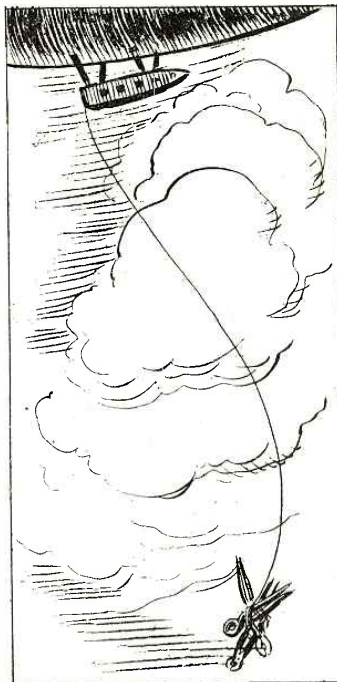
I Joined These Wires Together and Used Pliers for an Antenna Weight.
