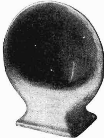
Fig. 5. A novel reflecting type of loud speaker, built of wood, which operated well.
