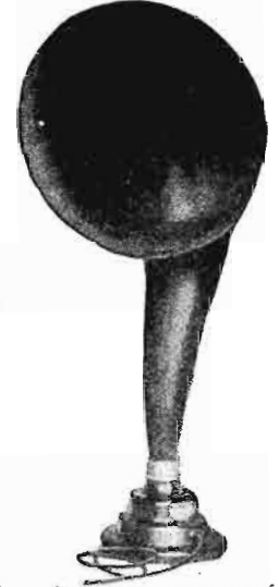
Fig. 4. Also a common type of horn loud speaker in which the horn itself is curved.
