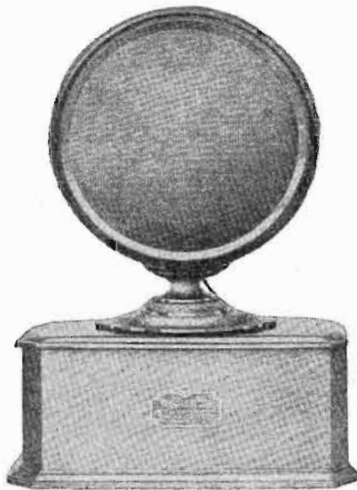
Fig. 7. A combined power amplifier and loud speaker that will provide ample volume for a dance hall.
