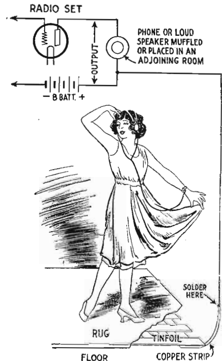
Fig. 3. Electrical connections showing how tinfoil under the rug is connected with the output of a multi-tube radio set. With some sets it is necessary also to ground one connection; the phone may be muffled, or the cap and diaphragm taken off, as shown in Fig. 4.
