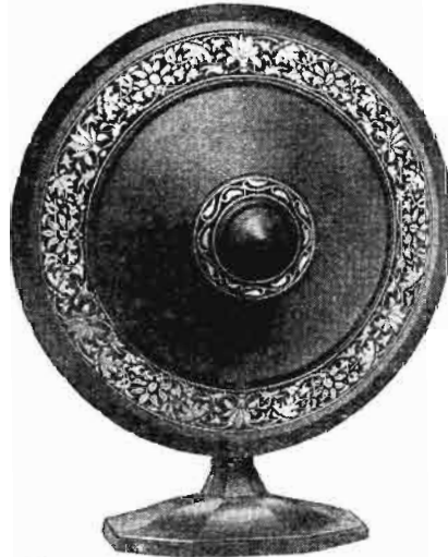
Fig. 6. A new type of cone loud speaker of free-edge construction, giving excellent reproduction.
