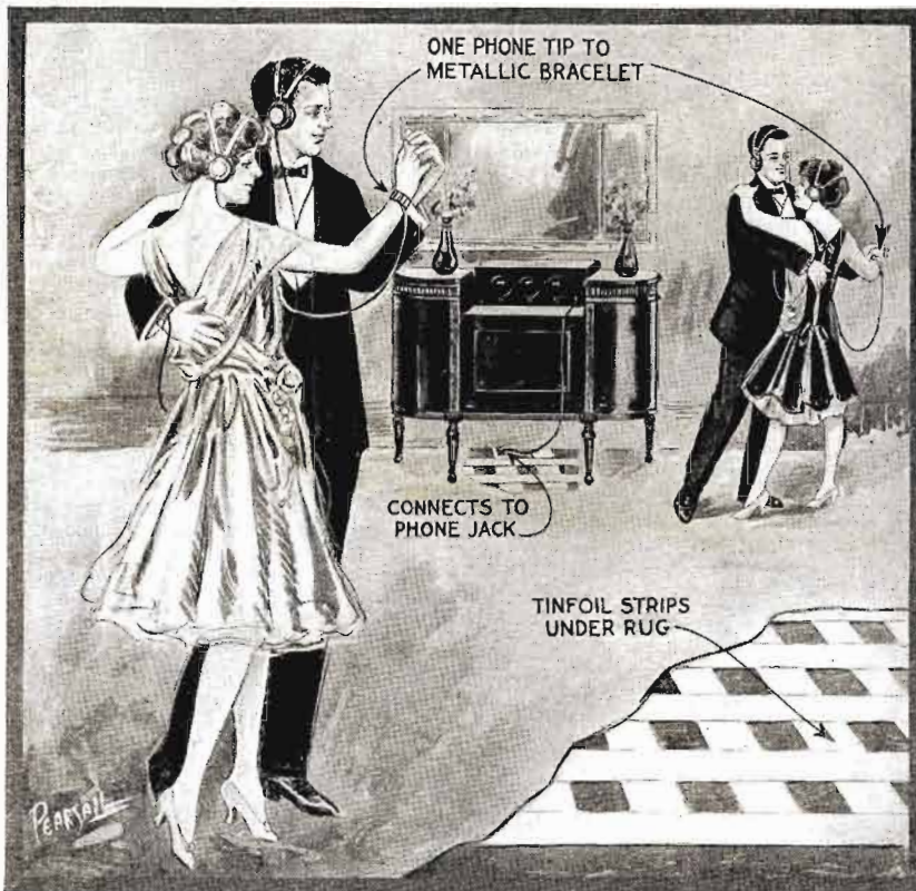
The secret of the wireless radio dancing exposed. Tinfoil strips are placed under the rug, while the cord that usually goes to the loud speaker is connected to the tinfoil. The dancers wear metallic bracelets on which one tip of the headphones is grounded. The concert comes through loudly and clearly as soon as the stations are tuned in.
