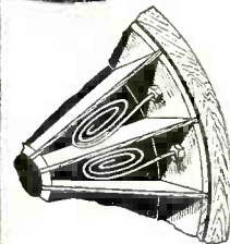
Two English loud speakers. That at the left is a cone-type with amplifier, complete in the cabinet. Above is the baffle, which has radial baffles in the cabinet.
