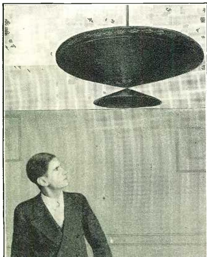
This shows how the illuminated double-cone speaker is suspended from the ceiling of a room, to act as a diffusing reflector. The electric light is within the hollow of the large cone, and is not visible in this view.
