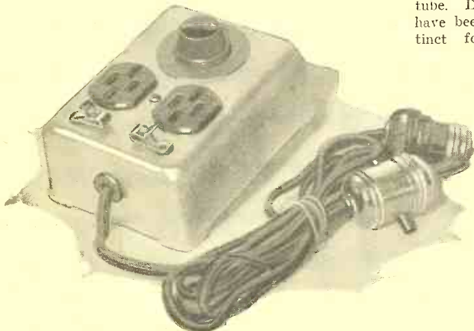
Fig. A The all-purpose lighting receptacle, power supply and antenna described above. Every external connection of a receiver is here provided for.
