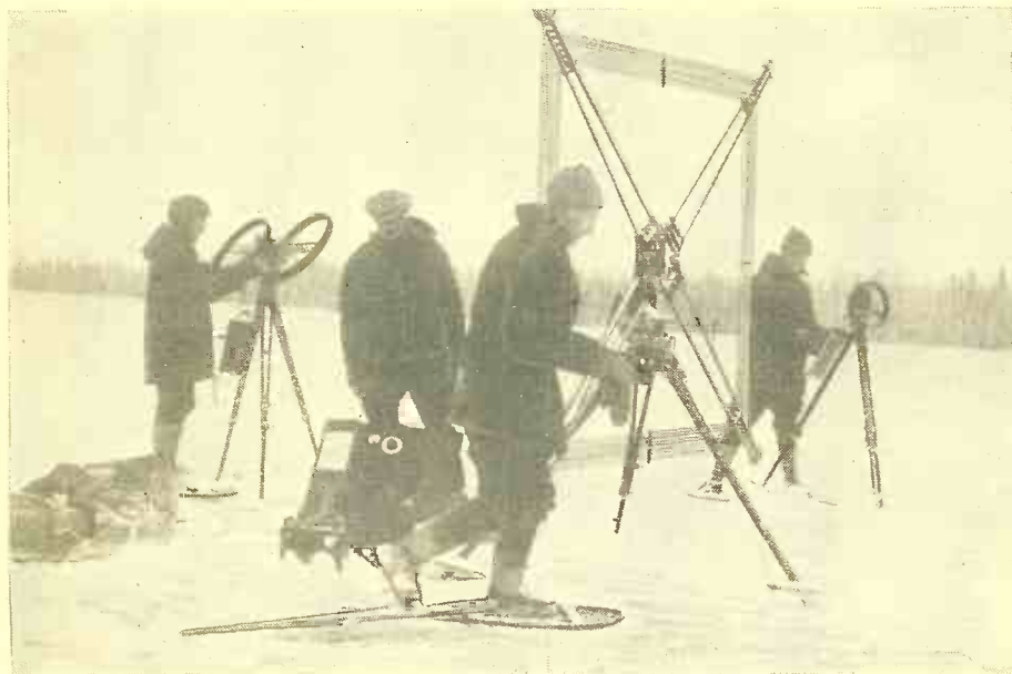
Here is a company of radio prospectors snowshoeing over a frozen lake in the north, carrying with them a quantity of their paraphernalia. The large loop is that of the transmitter, and the double hoops are those of receivers. (Photos courtesy The Radiore Company.)
