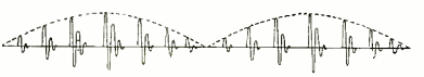
Approximate Variation in the Wave Train Amplitude During One Cycle. Only a Few of the Wave Trains are Shown for Clearness.
