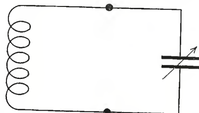
Fig. 1. The manner in which the coils and variable condenser are connected.
