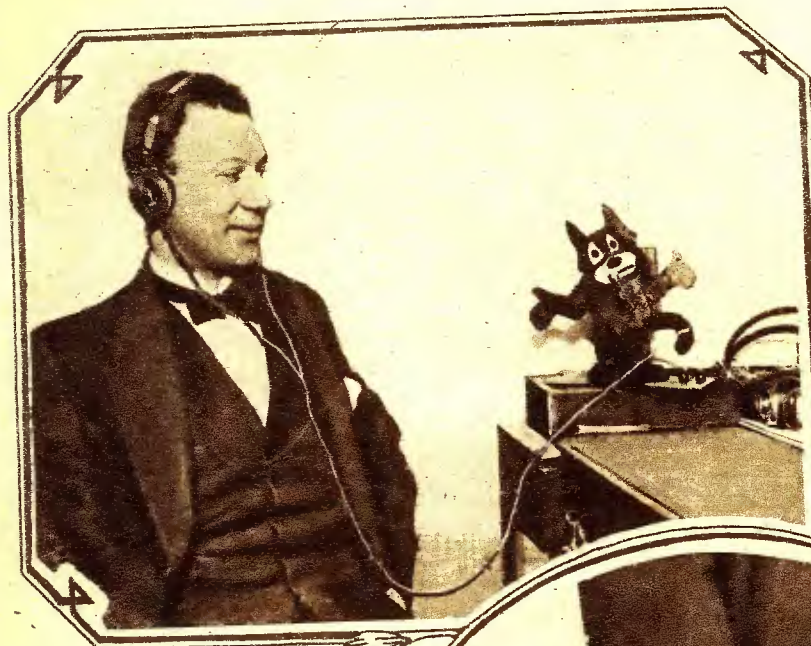
Above: A new feature in radio sets is this one of Pelix, the Movie Cat. The tail forms the tuner and the solitary whisker on the face acts as the "cat whisker" for the crystal. © Keystone View Co. Right: A complete radio receiving set that fits the vest pocket. The crystal detector is mounted on the small panel containing the switch. Below: A miniature honeycomb coil tuner that operates just as well as a large one.
