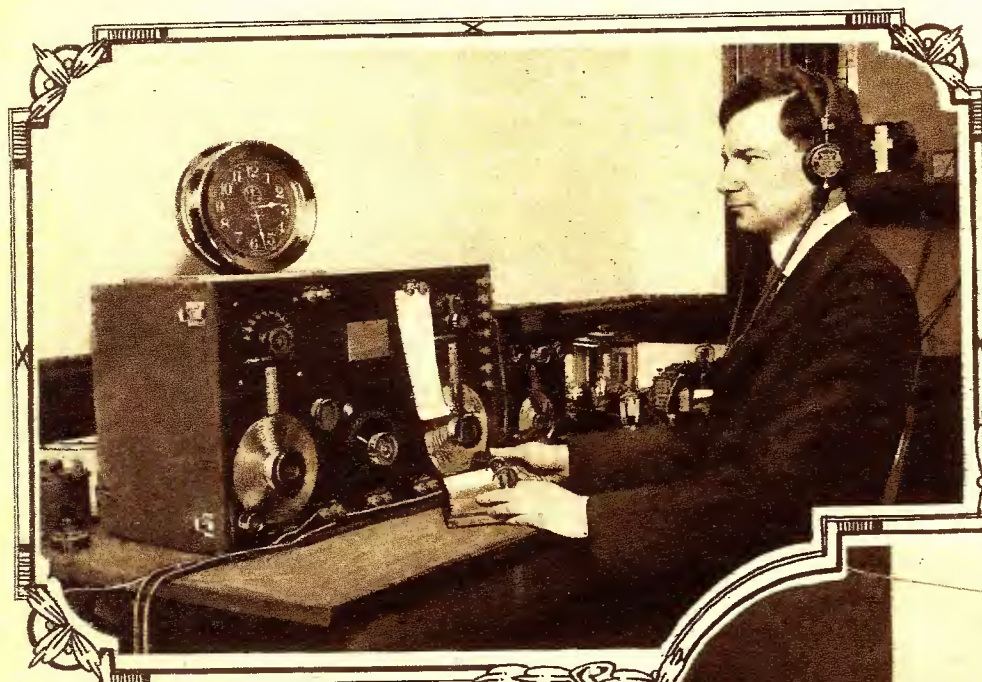
Left: Here is Paul Sollenburger, the man who attends to the transmission of the time signals from the U. S. Observatory at Washington, D. C. The signals are relayed from Washington by wire to the transmitting station, NAA at Arlington, Va., which works on a wave-length of 2,650 meters. This is a very powerful station and the time signals transmitted at noon and at 10 P.M. are heard by ships in both the Atlantic and Pacific oceans. No matter where you live, you have no doubt heard the time signals from NAA re-transmitted from some broadcast station. © Harris & Ewing
