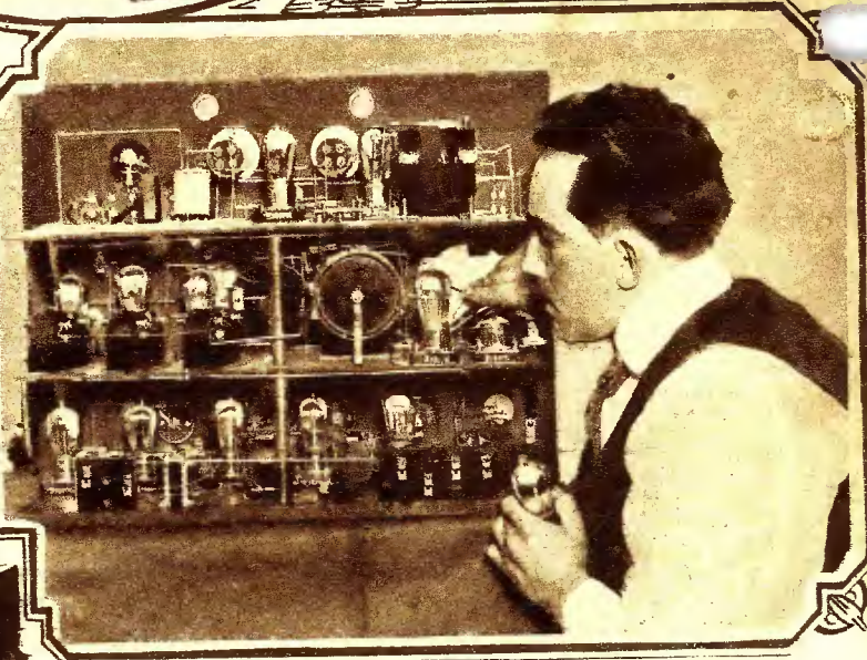
Above: This unique Super-Heterodyne was built by Henry Brinkman of Pelham, N. Y. The top shelf contains a two stage tuned radio frequency amplifier, the second shelf the detector, oscillator and intermediate radio frequency amplifiers, and the third shelf the second detector and three stages of audio frequency amplification, the third being push-pull. ©Kadel & Herbert. Left: John Shepherd, 3rd a prominent merchant of Boston owns this six tube portable radio set. It is composed of three stages of radio frequency amplification, a detector and two stages of audio frequency amplification. © International Newsreel.
