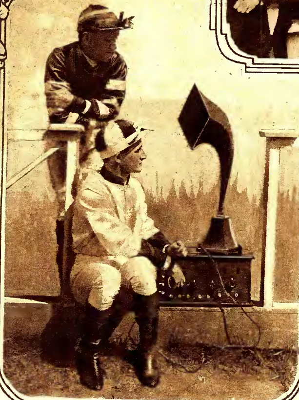
Left: Jockey Burns tunes in for Thurber just before the races at Belmont Park. The set employs two stages of radio frequency amplification, a detector and two stages of audio frequency amplification. © Foto Topics, Inc.
