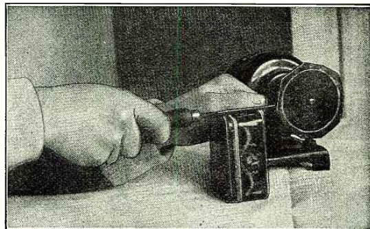
A good looking dial may be made from the hard rubber of an old battery jar.
