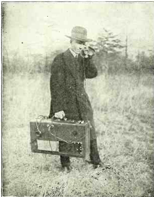
This Complete Receiver in a Suitcase Will Bring in Loud Stations Ten Miles Away, While Distant Stations Can be Heard With the Phones.
