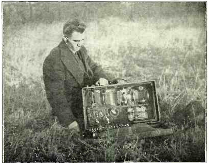
This Complete Receiver in a Suitcase Will Bring in Loud Stations Ten Miles Away, While Distant Stations Can be Heard With the Phones.
