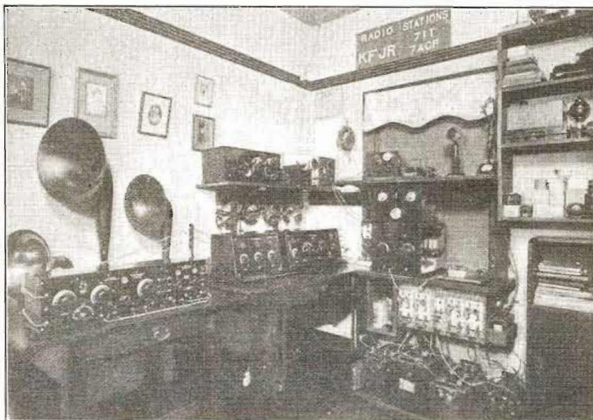
Station 7IT, 7ACP owned and operated by Ashley C. Dixon, Stevensville, Montana. His station is located in a valley and without commercial "juice." A 12-volt storage battery drives a 500-volt, 100-watt Dynamotor, which furnishes the pep for the 10-watt C.W. transmitter. This station has been heard in London, England, a distance of about 5,500 miles and has been reported at 1,500 miles on five watts.
