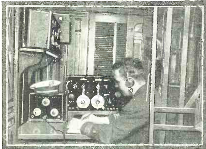
Above is Chief Radio Operator Orth at the "Macom's" receiver. At his left is a 5-tube superheterodyne with a power amplifier; at his right hand a navy type receiver, which has a range of 250 to 3,000 meters for receiving ship and land messages. In the picture in the upper right corner of the page, Mr. Orth is shown at the transmitting panel of the "Macom's" equipment. This is a 500-watt quenched-spark transmitter, and operates on 600 and 730 meters.
