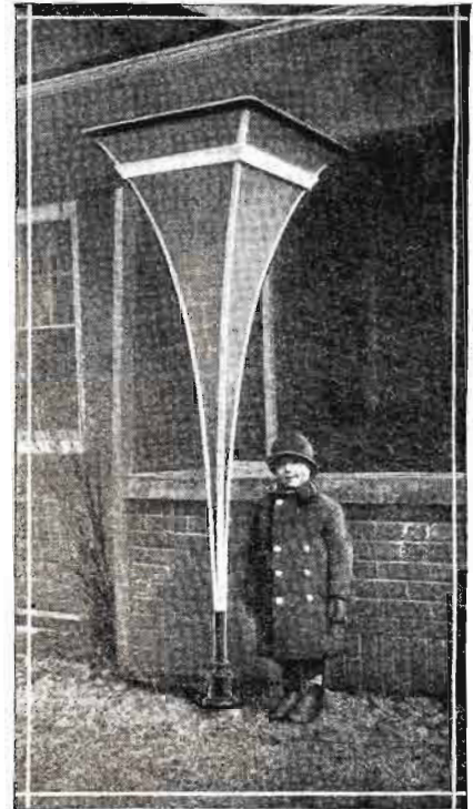
The extension of the exponential horn is the part above the white band near the top; its construction is described here.
