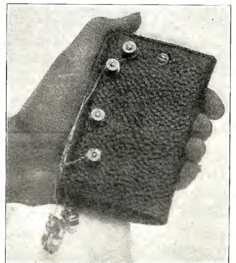
This Shows the Size of the Set When Folded. Two of the Binding Posts are for Aerial and Ground, the Two Others for the Fones.
