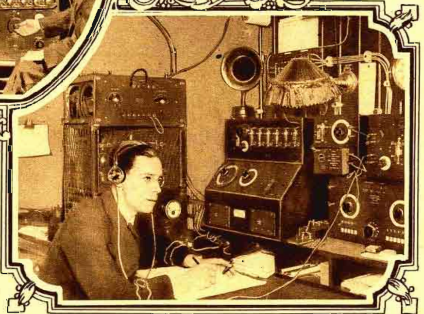
Above is a view of the radio room on the new S.S. Voltaire , one of the liners which plys between New York and South American ports. The C. W. transmitter to the left has an output of 1½ K.W., which insures an ample transmitting radius. In front of the operator is a six-tube direction finder and next to it, the receiving set which employs a separate heterodyne for the reception of C.W. signals. © Keystone View Co.
