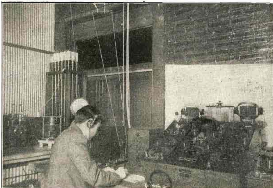
One of the old-time commercial stations that had apparatus built like a battleship, much better in fact than some of the present-day stuff. Note the two DeForest audions perched atop the left-hand receiving set. Also the large transmitting condensers in the rack by the window.
