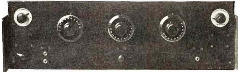
A front view of the Neutrodyne receiver built by Mr. Cushman. Note the positions of the jacks and rheostats.
