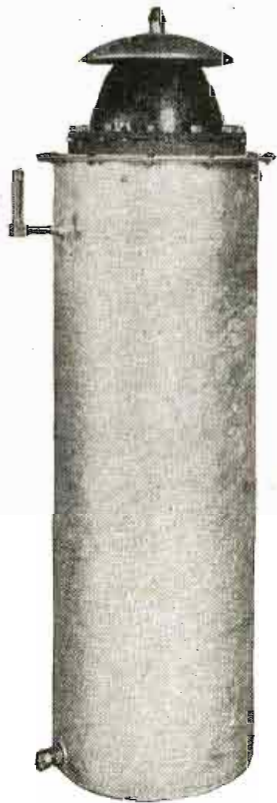
Fig. 24 This condenser built for the Navy Department to be used with a 30-K.W. arc transmitter can withstand 90,000 volts. It has a capacity of .002 MF. and is about 5 feet high.
