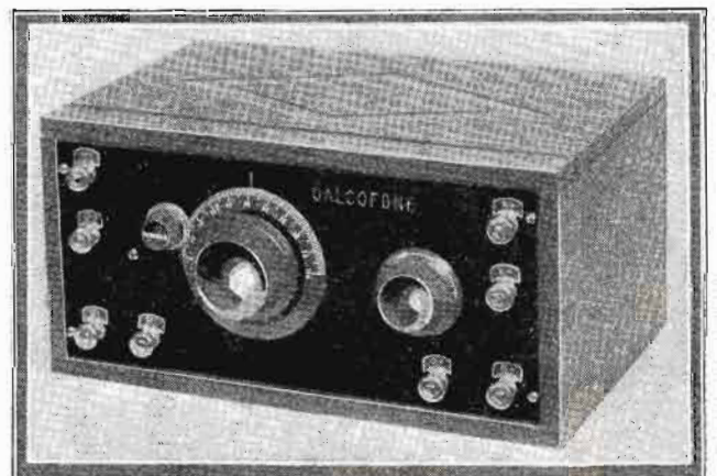
Fig. 5. A single-tube set, for the radio beginner who does not desire to invest much money in radio, is shown at the right. Under good reception conditions, this set will give exceptional results, considering the amount of equipment used.
