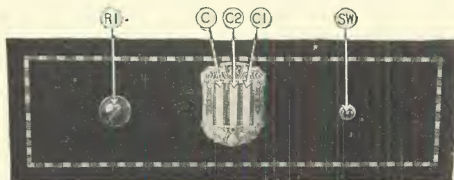
Front panel view of the Phasatrol-Balanced receiver. R1 is the volume control, SW the filament switch and C, C1 and C2 the tuning condensers. Note that condenser C2 (shown in the view at top of page) is controlled by the center drum.
