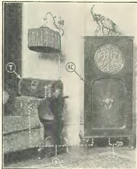
How the radio tuner and detector is connected to the audio amplifier and loud speaker.
