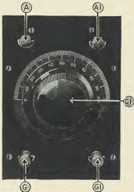
Fig. 15. A front view of the wavetraps, the circuit of which is shown in Fig. 4-A. Note that there are two aerial and two ground posts. Photo courtesy of X-L Radio Laboratories
