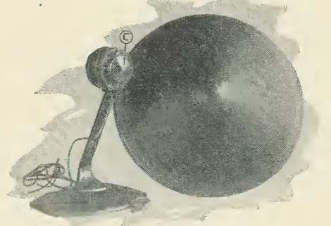
The paper cone has been removed from the stand, in this view, to show the position of the driving cone C, to which the paper is fastened by a single nut.
