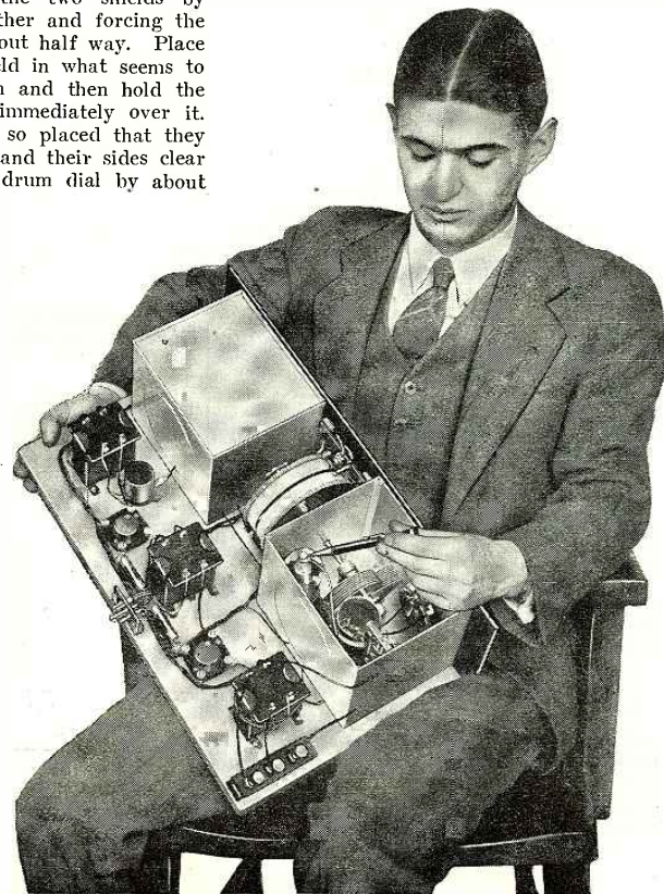
The shield-top of the R.F. amplifier stage removed, with the pencil indicating the top terminal of the screen-grid tube.
