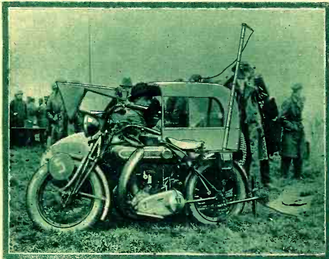
In the above illustration is pictured a new French military motorcycle and side-car, which is equipped with a complete transmitting and receiving station. On the rear of the machine may be seen the bamboo pole to which is attached the antenna. The apparatus, which is under the hood at the back of the side-car, is operated from a seat at the front of the car. The apparatus is shown undergoing army tests.
