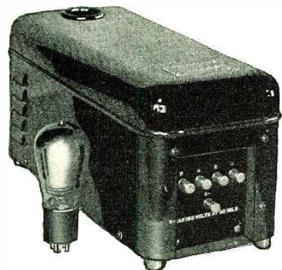
Outside view of the "B" socket supply unit, showing the terminal strip and the rectifier tube.
