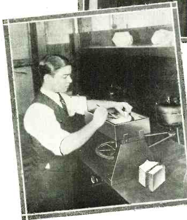
Below, the process of grinding the quartz crystal to the exact thickness required. This is a very delicate operation, which may be compared with work on a lens. The thickness of the crystal regulates its frequency.
