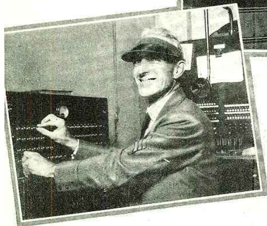
Sergeant on duty at police headquarters at Berkeley, Calif., under his hand buttons each of which will light a red signal in a patrolman's car. He can thus send a flashing signal in Morse code; or direct the patrolman to listen in through phones or turn on his loud speaker.
