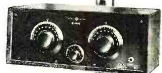
FADA Neuro Junior No. 195 Three-tube Neutrodyne. A wonderful performer. Price (less tubes, batteries, etc.) $75.
