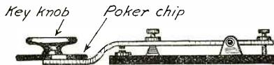
A poker chip transforms an ordinary key knob to one of the Navy type.
