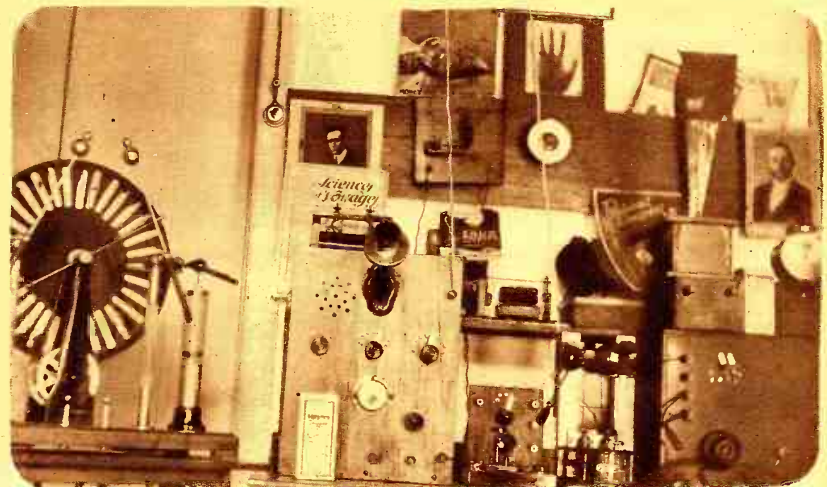
The amateur station owned and operated by Augusto J. Pereira, Pernambuco, Brazil. The transmitter employs one 5 watt tube. Plate voltage is secured from "B" batteries. Absorption modulation is employed for fone work. The receiver of the Honeycomb coil type has a wave-length range of 350 to 20,000 meters. A 6-wire fan shape counterpoise is employed in conjunction with the transmitter. All of the apparatus is home made.
