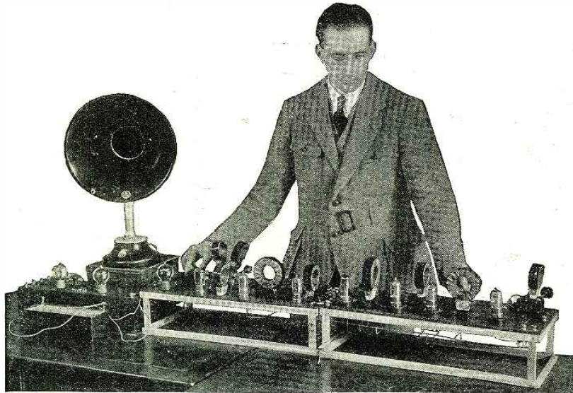
The author experimenting with a ten tube multi-stage radio frequency receiver. The system employed is fully covered in this article.
