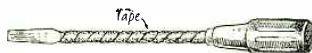
By wrapping a layer of tape around the screw driver, the danger of short circuits is eliminated.
