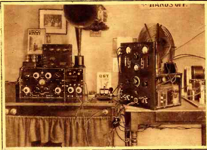
Station 9DCP, owned and operated by H. M. Degolier, London, Wis. The aerial, a four wire inverted L with caged lead-in, is supported by a 100-foot steel tower at one end. The counterpoise 14 wires in fan shape, is 20 feet above ground. The C.W. transmitter employs two 50-watters in the 1DH circuit, using rectified A.C. on the plates. The phone set employs a 500-watt oscillator, 50 watt modulator and a 5-watt special amplifier. The receiver is a Kennedy set.
