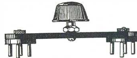
Two vacuum-tube bases provided the prongs used in this cable connector, which won seventh prize.
