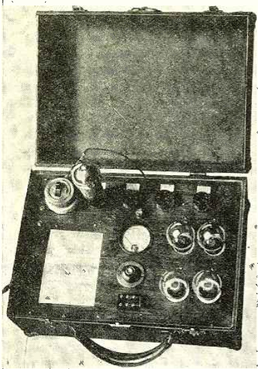
Mr. Shaffer's handy tube tester, ready for immediate use, in its carrying case
