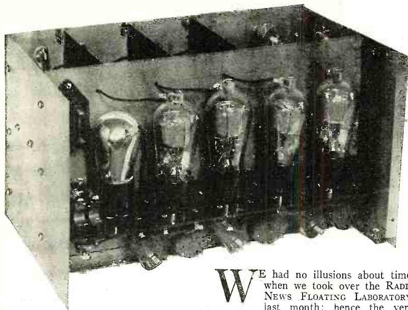
A rear view of the experimental receiver, with top and back removed. Above—using the trouble finder in making interference tests on board
