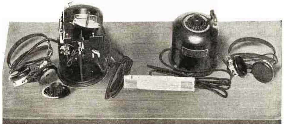
Fig. 2. Assembled and unassembled views of the wired radio crystal receiver. The long flexible wire has a plug on the end which is screwed into any lamp receptacle in the house when it is desired to receive.
